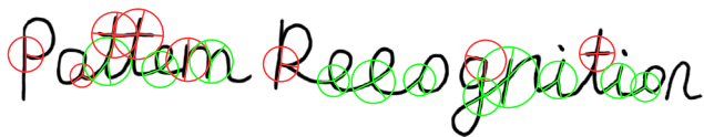
Fig. 2. Junctions in handwritten characters. The junctions marked in light (red) are within a character itself, and the green ones are from stroke touching. (For interpretation of the references to color in this figure caption, the reader is referred to the web version of this paper.)
