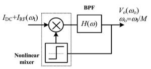
Fig. 4. Nonlinear feedback model for the injection-locked frequency divider.
