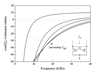
Fig. 3. Real-part impedance performances of the cross-coupled circuit depending on  $V_{DS}$ . ( $V_{DS}$ =0.2 V $\sim$ 1 V, step 0.2 V).
