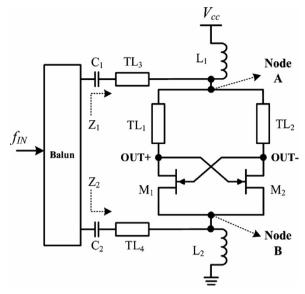
Fig. 1. Schematic diagram of the differential-injection ILFD.
