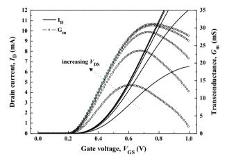
**Fig. 2.** Drain current  $(I_D)$ /transconductance  $(G_m)$  characteristics versus gate and drain biases  $(V_{DS}=0.2 \text{ V} \sim 1 \text{ V}, \text{ step } 0.2 \text{ V})$ .
