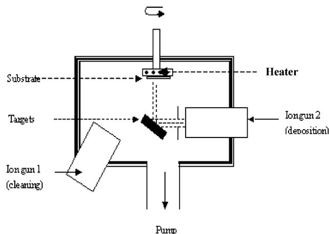
Fig. 1. The schematic diagram of ion beam sputtering instrument.
