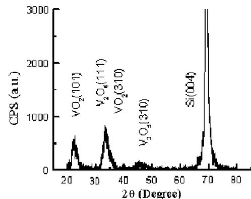
Fig. 2. The XRD pattern of the as-deposited samples under lower O<sub>2</sub> pressure ( $1 \times 10^{-3}$  Pa).
