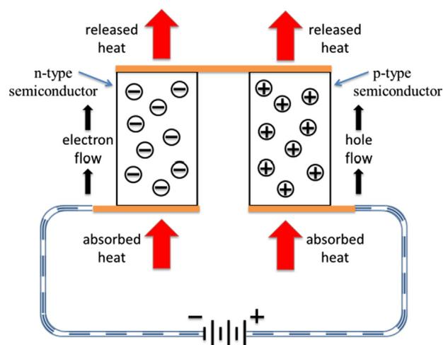
Fig. 1. Working principles of TEC.
