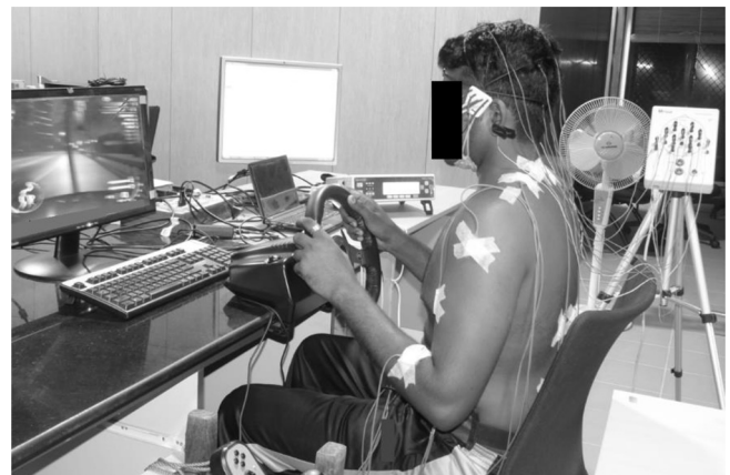
Fig. 1. Experimental setup includes driving simulator, data acquisition systems for surface electromyographic and electroencephalographic signals, seat interface pressure mapping system and photoplethysmography unit for heart rate and blood pressure monitoring.
