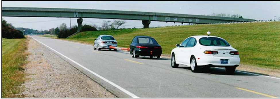
Fig. 1. The surrogate target lead vehicle methodology and test track employed in the Kiefer et al. (1999) study.
