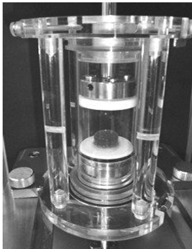
Fig. 1. Instrumental mastication simulator to prepare model bolus.
