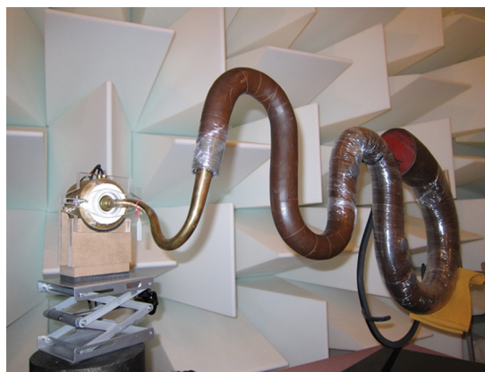
Fig. 2. Experimental setup used to measure the input impedance of historical serpents.
