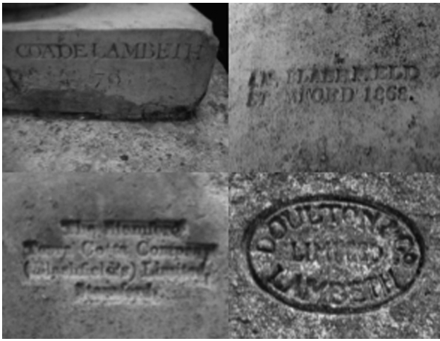
Fig. 1. Examples of manufacturer's stamps on ceramic objects. Clockwise from the top left: Coade Lambeth 1779 (AACA, AACB, AACC); J.M. Blashfield Stamford 1868 (CABA, CABB, CABC); The Stamford Terra Cotta Company (Blashfield) Limited, Stamford (1872–5) (BA, BC); Doulton & Co Ltd Lambeth (1890–1902) (CADA, CADB, CADC, CADD).
