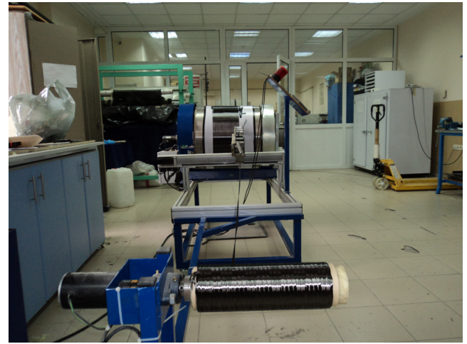
Fig. 1. The production of the prepreg composite.
