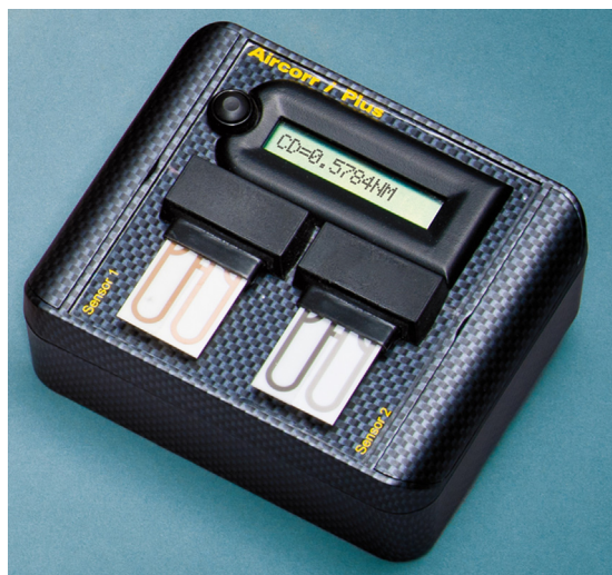
Fig. 1. AirCorr corrosion monitoring system equipped with Ag-50 nm and Cu-50 nm sensors.
