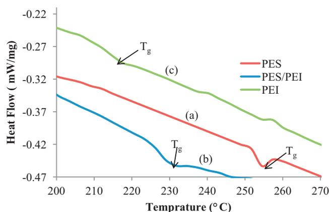
**Fig. 1 – DSC thermograms of the membranes prepared from PES (a), PES/PEI with blend composition of 92:8 (b) and PEI (c).**
