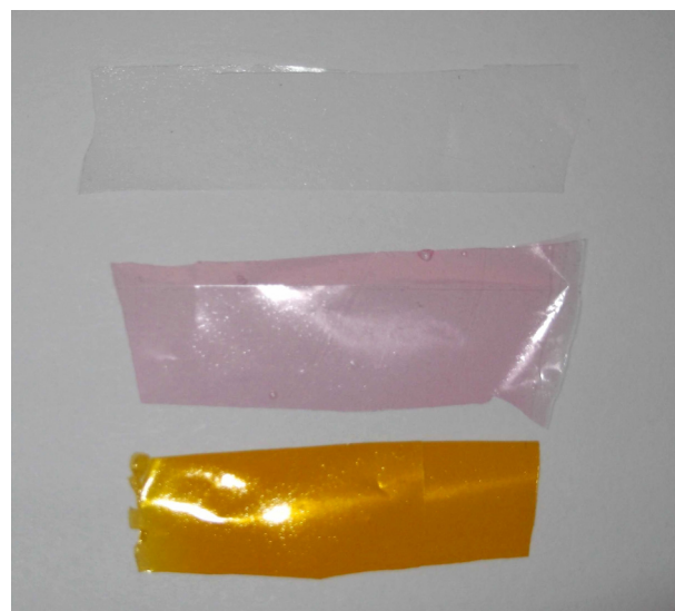
Fig. 1 – Thin dry films: pure HPMC, methyl orange in HPMC (yellow) and Vitamin B12 in HPMC (pink). (For interpretation of the references to color in this figure legend, the reader is referred to the web version of the article.)
