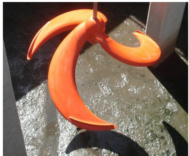
Fig. 2 – Philadelphia Mixing Solution Ltd. XELSC-2200 high efficiency anti-ragging impeller developed in 2008.
