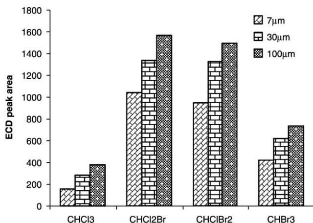
**Fig. 1.** Extraction efficiencies with different film thicknesses of the PDMS fiber: extraction time of 20 min at 35 °C, desorption time of 4 min at 250 °C. THM concentration: 80 µg/l,  $n = 5$ .
