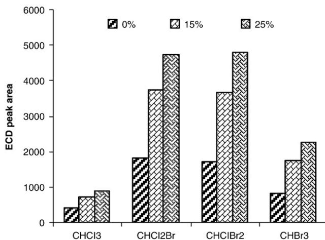
**Fig. 2.** Effect of the addition of salt and magnetic stirring on extraction: extraction time of 20 min at 35 °C, desorption time of 4 min at 250 °C. THM concentration: 80 µg/L,  $n = 5$ .
