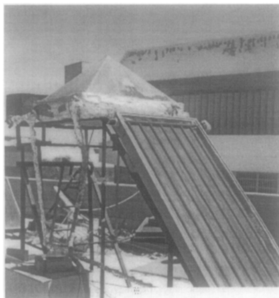
Fig. 1. Photograph of the still-collector system.
