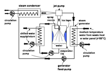
Fig. 1. Showing the proposed jet-pump - thermal ice storage system.
