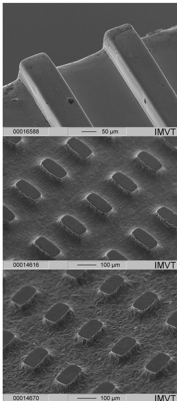
Fig. 1. Stainless steel microstructure foils to be integrated into crossflow heat exchanger devices. Top–down: Micro-channels arrays, linear micro columns, staggered micro columns. All microstructures have been made of stainless steel.
