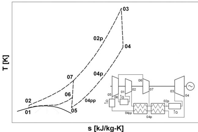
Fig. 2. T–S diagram of the supercritical carbon dioxide cycle (layout 2).
