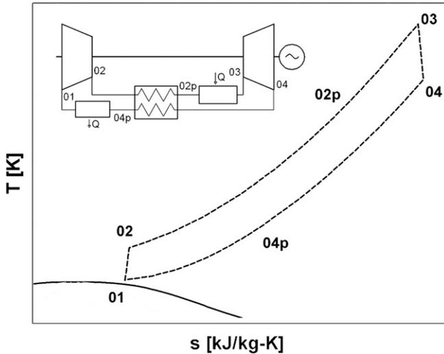
Fig. 1. T–S diagram of a simple recuperative carbon dioxide topping cycle (layout 1).
