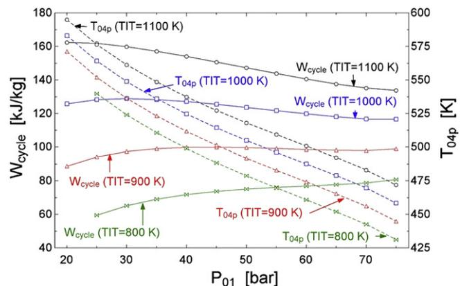
Fig. 3. CO<sub>2</sub> cycle (layout 1). Effect of compressor inlet pressure (P01) on specific work and recuperator hot delivery temperature ( $T_{04p}$ ). Carbon dioxide cycle (layout 1).
