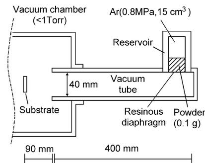
Fig. 1. Schematic illustration of the spray deposition technique.
