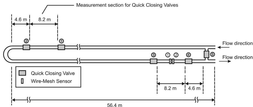
Fig. 1. Schematic layout of the 6-inch low-pressure flow loop test section.
