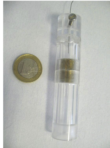
Fig. 1. Diagram and photograph of electrostatic actuator and sampling device.
