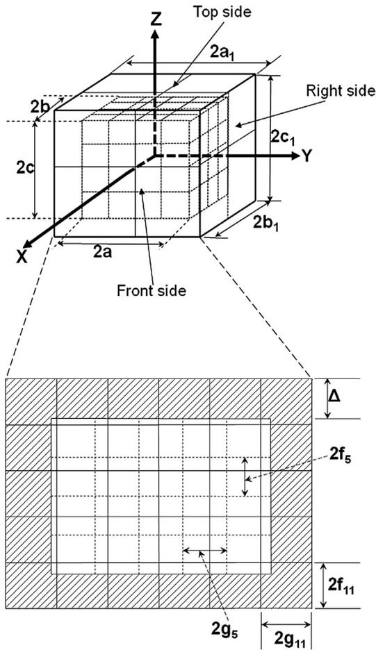
Fig. 1. Dielectric coated parallelepiped with expanded front side.
