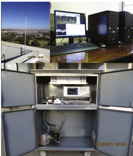
Fig. 1. Physical spectrum measurement system.
