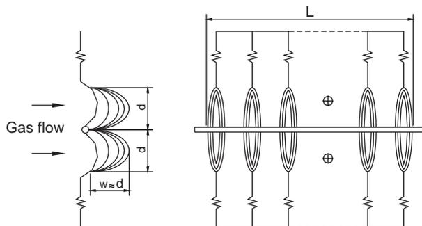
Fig. 1. Schematic diagram of the resistance ballasted multiple pins anode and tubular cathode.
