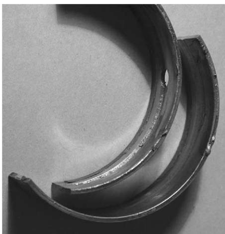
Fig. 2. Damaged main bush.
