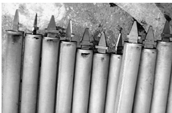
Fig. 2. Location of the defects near the top of the sintered cartridges.
