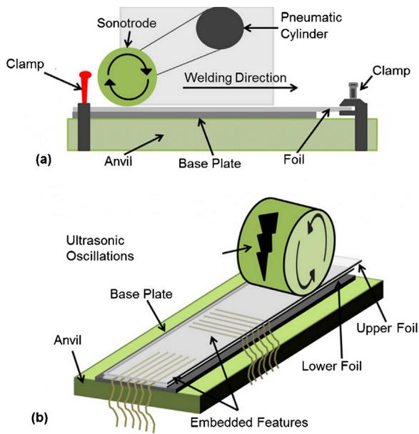
**Fig. 1.** Schematic overview of the Ultrasonic Consolidation process (a) front view and (b) embedding features.
