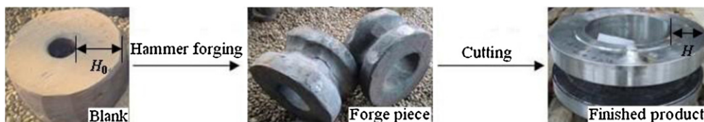
Fig. 2. Conventional manufacturing process of these rings.
