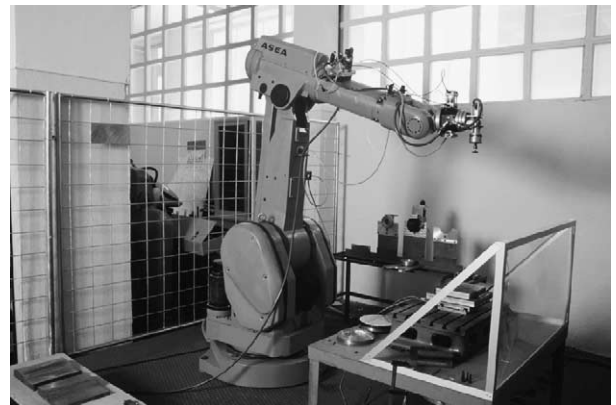
Fig. 1. Robot polishing cell experimental setup.
