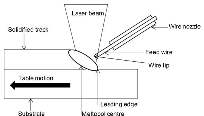
**Fig. 1.** Schematic representation of the laser deposition system.
