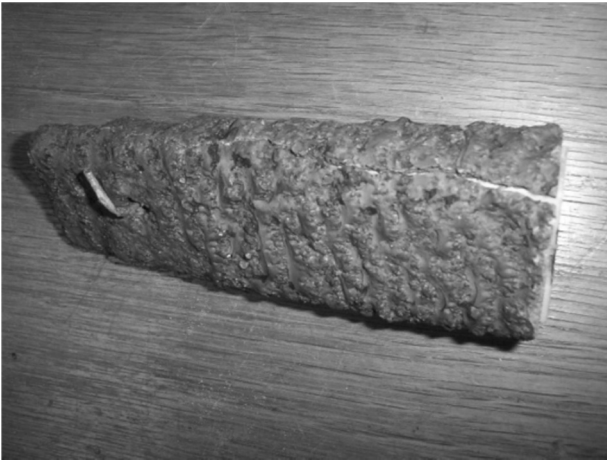
Fig. 1. Crack formed in shell during firing.
