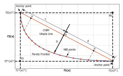
Fig. 1. Graphical description of NBI method.
