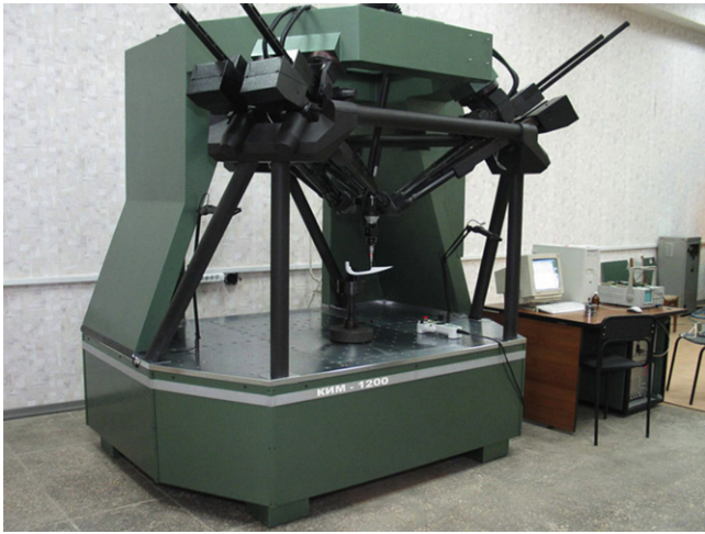
Fig. 1. A CMM of hexapod design. Courtesy of Laptic, Russian Federation.
