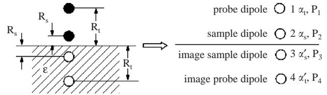
Fig. 2. Schematic diagram showing the image dipole model for SNOM, i.e. the probe tip dipole, the sample dipole and their image dipoles.
