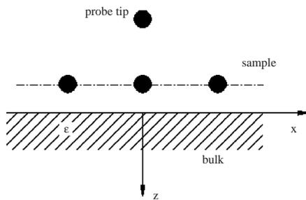
Fig. 1. Schematic diagram showing the geometry of system, i.e. the probe tip sphere, the sample in SNOM.
