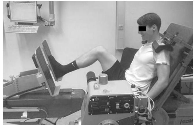
Fig. 1. Experimental setup. The subject is placed in the motor-driven leg press dynamometer (IsoMed 2000).
