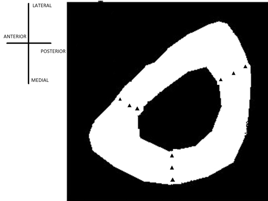
Fig. 1. Indents (black dots) distribution in the cross section of bone at the anterior, posterior and medial regions of a rat tibia.
