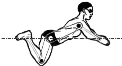
**Fig. 1.** A breaststroke swimmer modeled as two slider–crank mechanisms. Extremities are sliding back and forth along an axis (dash line) parallel to the surface, and animated from the center of the crankshaft (hip joint) through the cranks (thighs and trunk) and the connecting rods (lower legs and arms).
