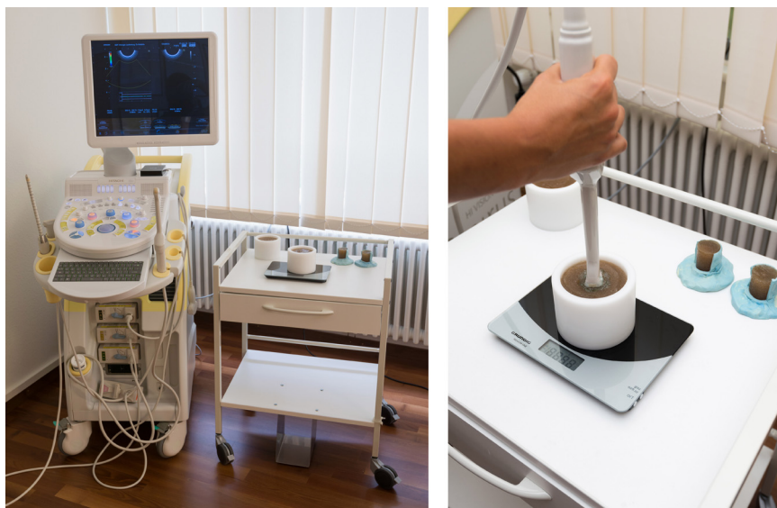
Fig. 1. Experimental setup for elastography measurements on phantoms using Hitachi VISION Preirus. Left: Hitachi ultrasound machine and test bench. Right: elastography measurement on phantom placed on balance.
