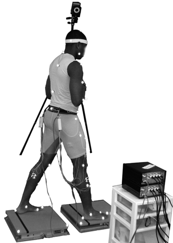
Fig. 1. Double support starting position for the study, with one foot on the front force plate and one foot on the back force plate.
