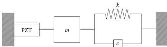
Fig. 1. Scheme of a 1-D electromechanical impedance model (adapted from Park et al. (2006)).
