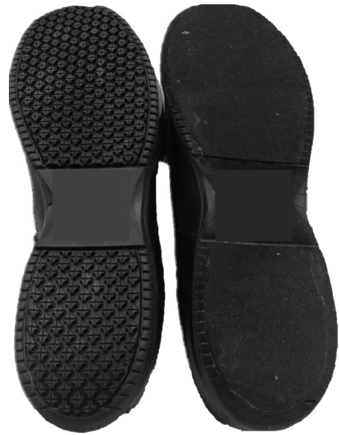
Fig. 1. Picture of the fully treaded shoes (left) and the untreaded shoes that had the tread fully removed (right).
