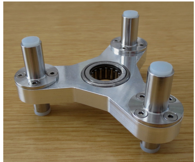
Fig. 2. Triple pin holder, shown upside down. Pin holder sleeves (press fit) are made from 316 L stainless steel (ASTM F138). Needle bearing has spherical housing which ensures uniform loading among pins.
