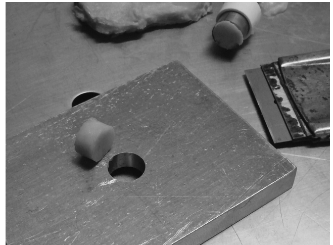
Fig. 2. The 12 mm punch, 6 mm aluminum plate and blade used for sample preparation.
