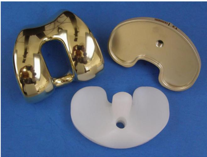
Fig. 1. Total knee arthroplasty device (AS Vega System<sup>®</sup> PS) with femoral and tibial components out of a CoCr29Mo6 alloy with a multilayer ZrN surface coating and a posterior stabilised gliding surface out of UHMWPE.
