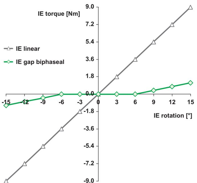
Fig. 2. Restraining AP shear force (left) and restraining IE torque (right) applied in the two test methods ISO<sub>linear</sub> and ISO<sub>gap biphasal</sub>.
