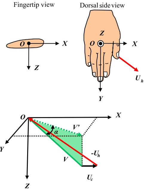
**Fig. 2.** Local coordinate system on the hand and definition of the angle of attack ( $\alpha$ ). The constant flow velocity vector of the main flow was  $U_c$  and the moving velocity vector of the center of the hand was  $U_h$ . Therefore, the resultant flow vector relative to the hand ( $V$ ) was the vector sum of  $U_c$  and  $-U_h$ . The angle of attack ( $\alpha$ ) was defined as the angle between  $V$  and its projection  $V'$  on the plane of the hand (the  $X$ - $Y$  plane).
