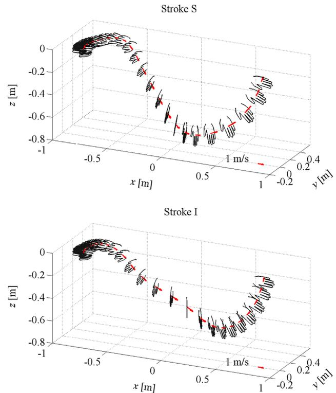
**Fig. 4.** 3D Hand trajectories for *Stroke S* (upper panel) and *Stroke I* (lower panel) at intervals of 125 ms. Red arrows represent the moving velocity vector ( $U_h$ ) of the center of the hand. (For interpretation of the references to color in this figure legend, the reader is referred to the web version of this article.)
