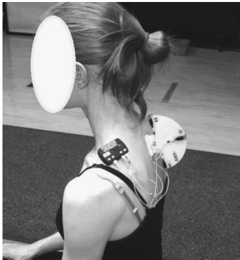
Fig. 1. Position of the CRCTM on a normal subject. The rigid cluster is made of lightweight plastic with a small rectangular base that is attached to the skin using double sided sticky tape. The mount is positioned proud of the back so markers are not obscured by shoulder or arm movement.
