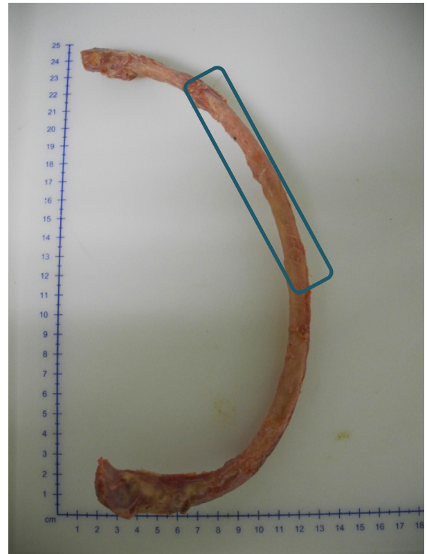
Fig. 1. The rectangle represents the location of the specimen (120 mm) cut from the rib.
