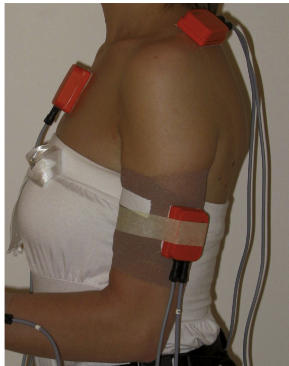
Fig. 1. Example of sensor placement for the ISEO protocol. For measuring the scapulo-humeral coordination, 3 sensors are required, positioned over thorax, scapula and humerus.
