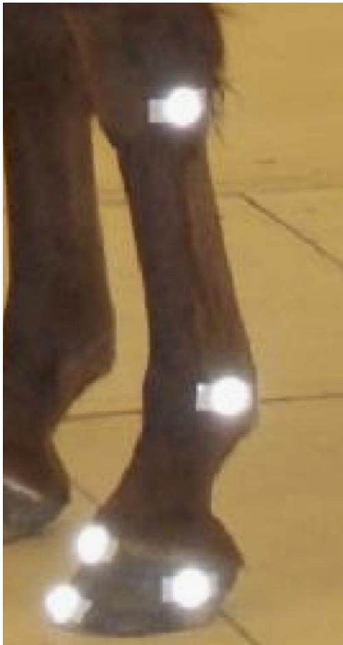
**Fig. 1.** Illustration of the marker placing on a horse from the trials. The markers on the Proximal metacarpus/metatarsus, on the fetlock joint and at hoof coronet are used in algorithm B for the detection of fetlock joint angle. The marker on the lateral hoof is used in method C and D. The distal dorsal hoof marker is used in method A, B and E to detect horizontal hoof speed and vertical acceleration.
